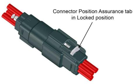
2) Once the CPA tab has been slid back, depress the locking latch. Push the connector slightly towards each other and then pull away from each other.
